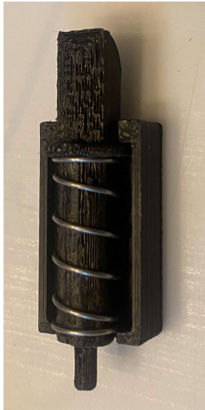
Figure 18: 3D Printed Latch Design
