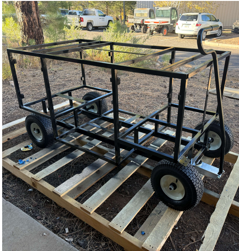
Figure 17: Raw Frame With Wheels
