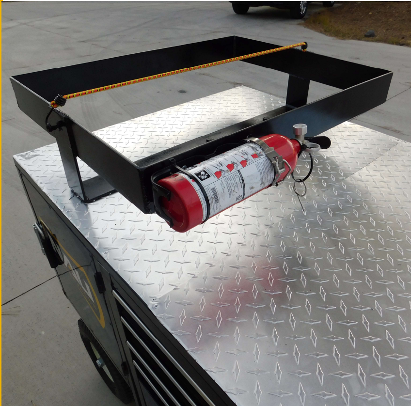
Figure 25: Mounted Tire Carrier/Extinguisher
