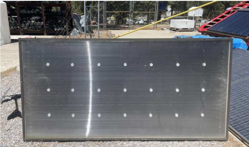
Figure 1: Air-Based Solar Thermal Panel
