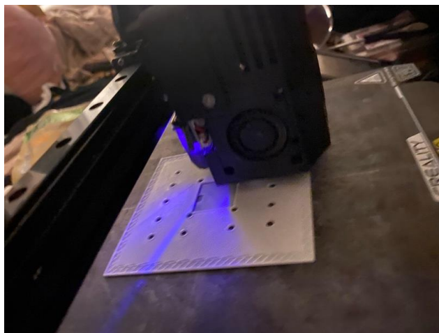
Figure 57: 3D Printing of TPU Casing
