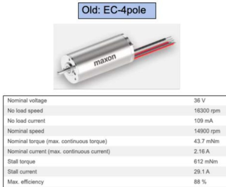
Figure 14: Factory Specifications of old motor without gearbox
