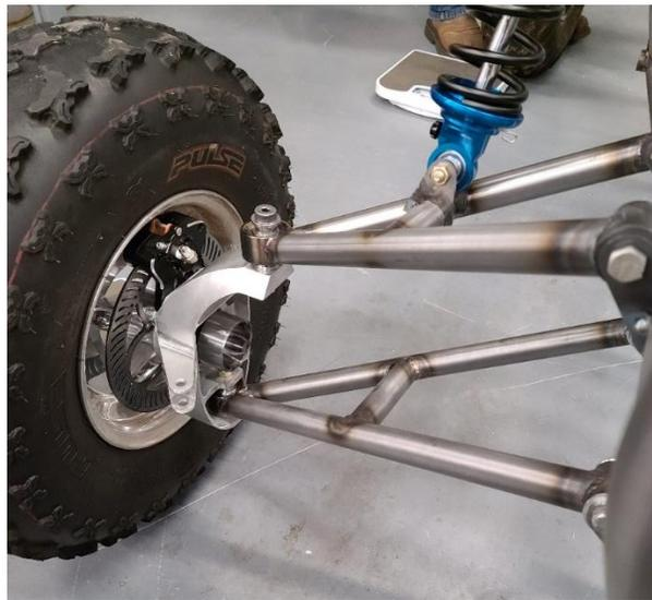
*Figure 28: Passenger Side Knuckle*
