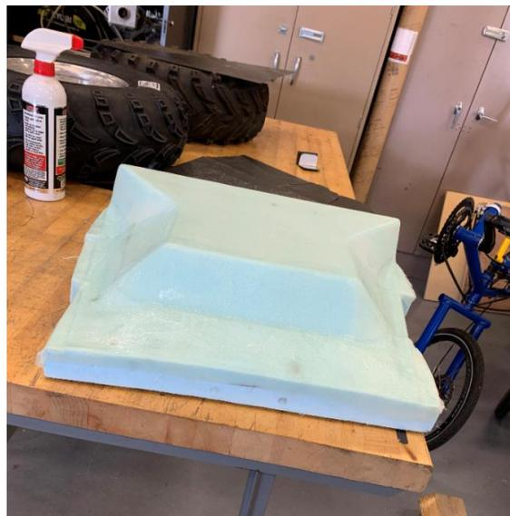
Figure 2: CNC Machined Fiber Glass Hood
