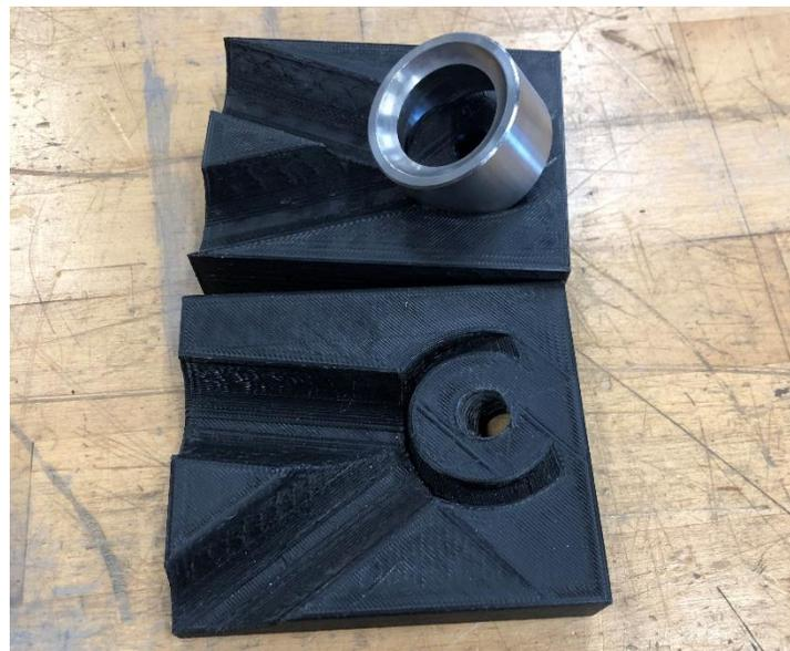
*Figure 23: 3D Printed A-arm Jigs*
