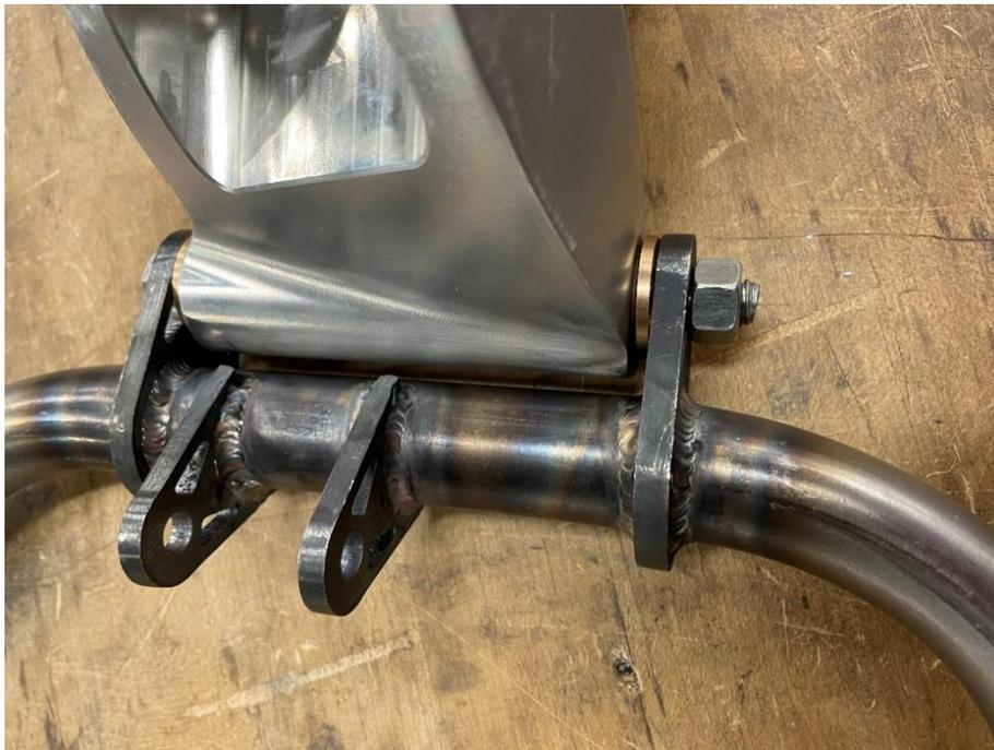
*Figure 30: Knuckle mounting Tabs*
