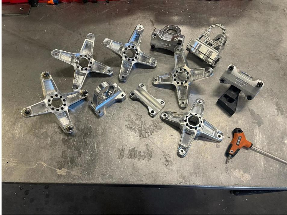
Figure 19: More Rear Hub and Pillow Block Bearing Clamps
