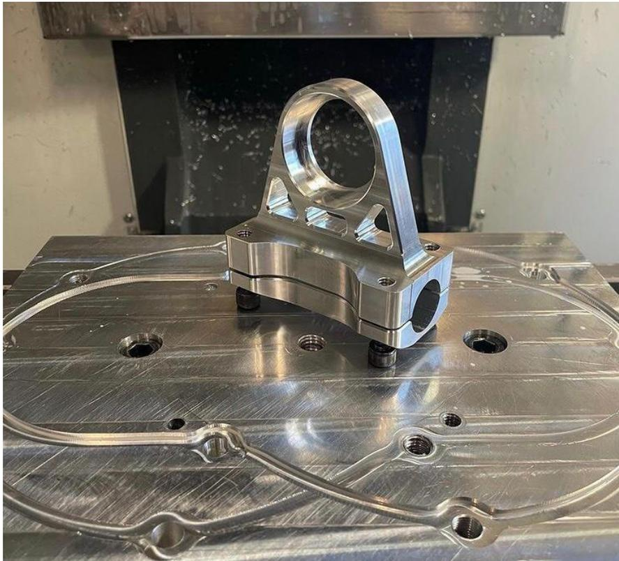
Figure 15: Pillow Block Bearing Clamp
