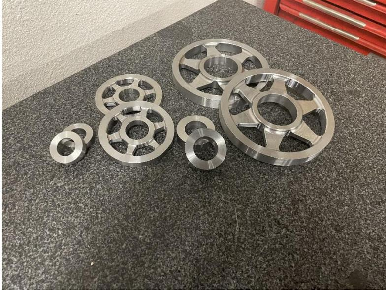
Figure 13: Gear Blanks Machined from 9310
