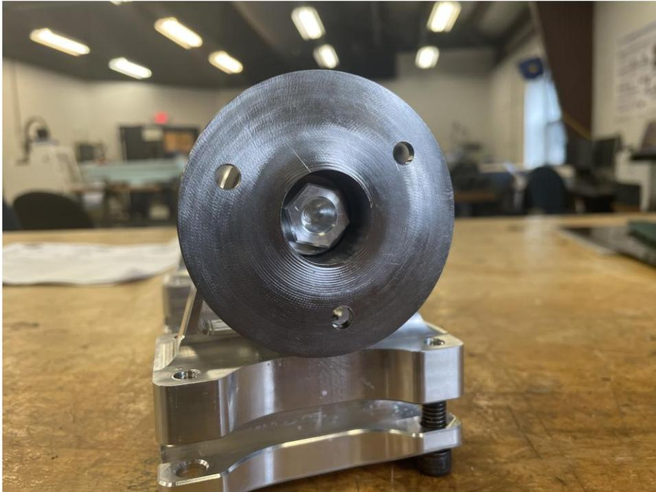
Figure 17: Front Half-Shaft Joint
