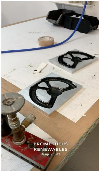
Figure 4: Nova Kinetics Facility, Steering Wheel Pre-preg Lay-out
