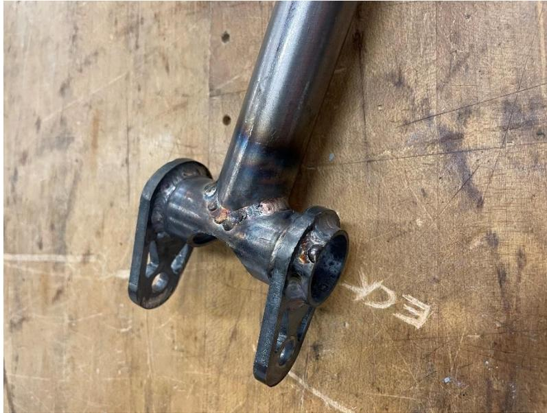
*Figure 31: Rear Arm Knuckle Mounting Tube/Tabs*
