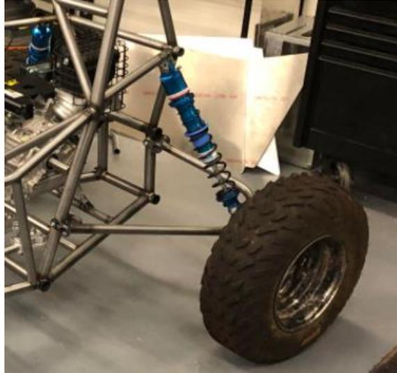
*Figure 33: Rear Suspension Mockup*
