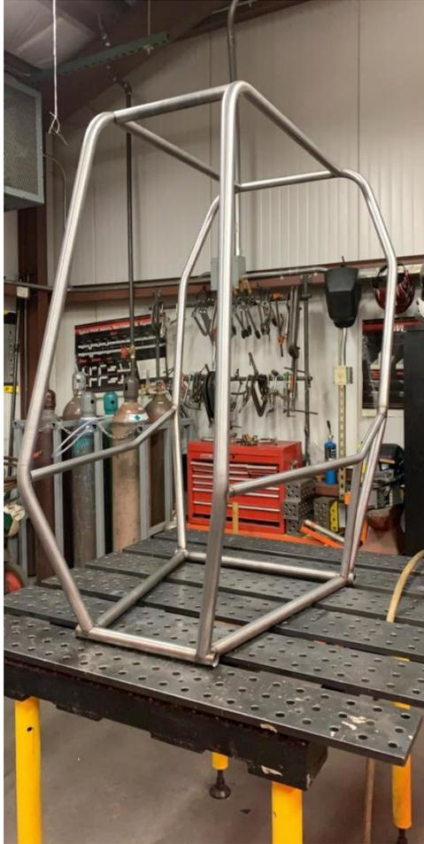
Figure 1: Isometric view of Primary Members tack-welded together
