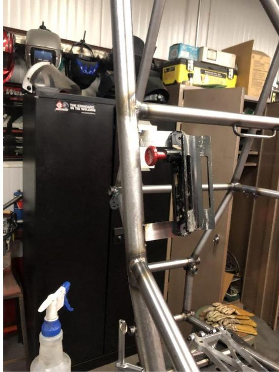
Figure 7: Fire Extinguisher Mount
