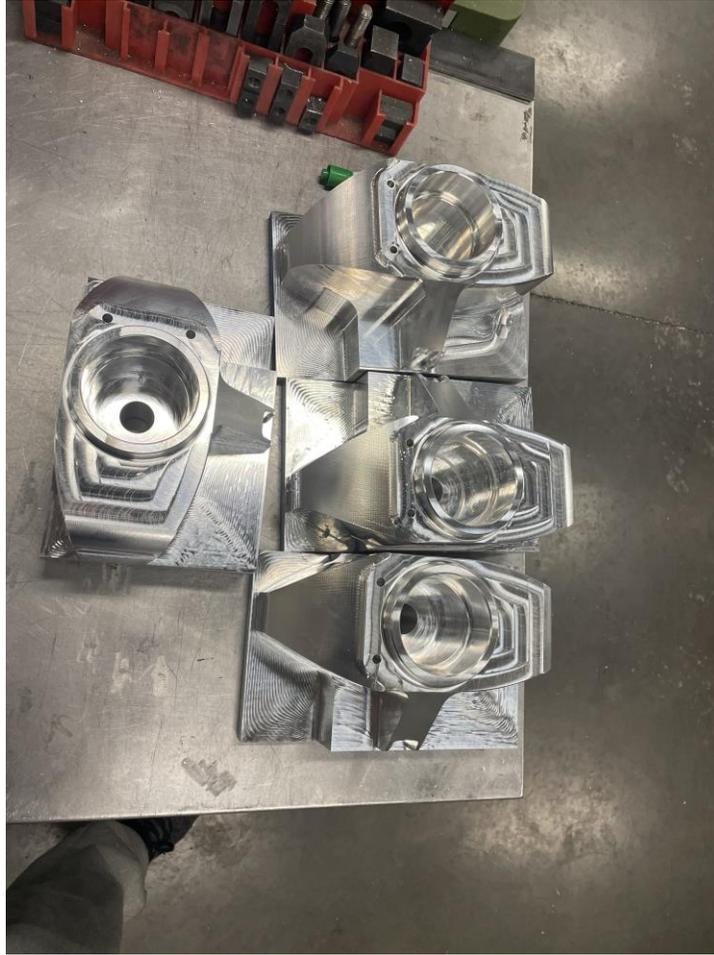
Figure 10: Front Upright's Left and Right Sides
