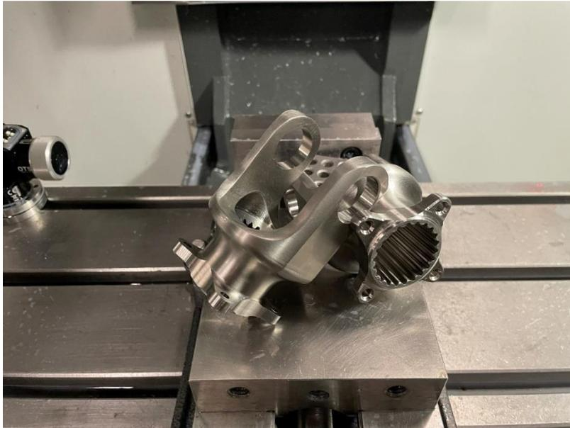
Figure 12: U-joint yokes machined from titanium
