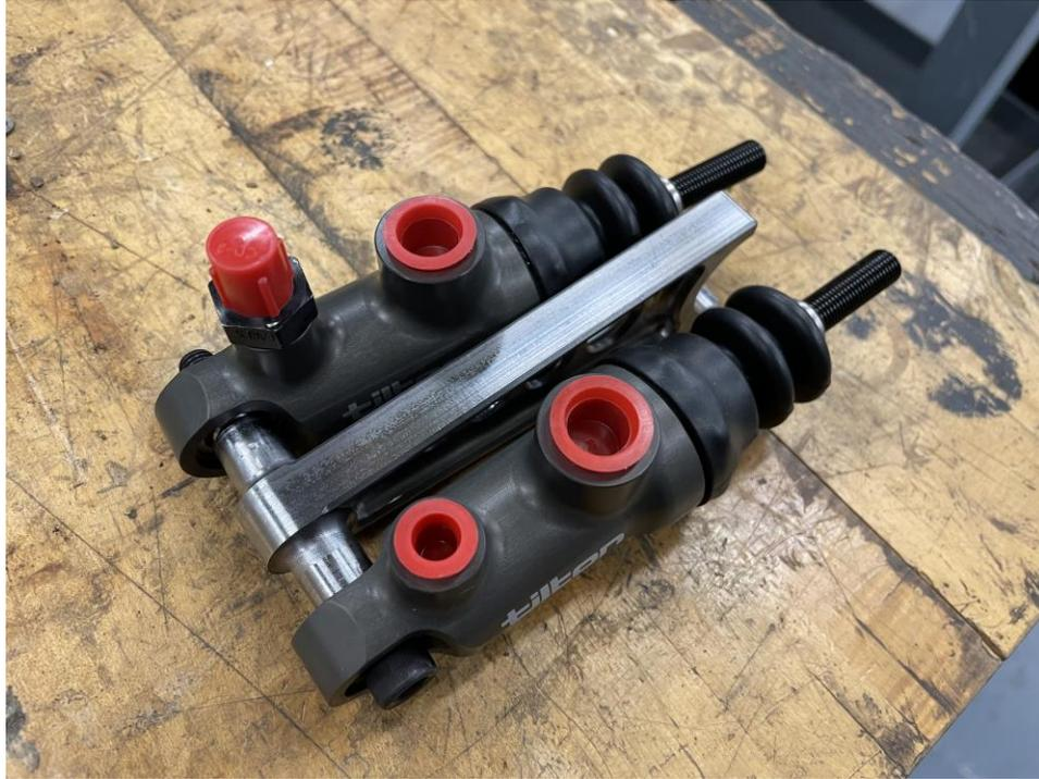
Figure 11: Master Cylinder Mount machined from 4130uyb
