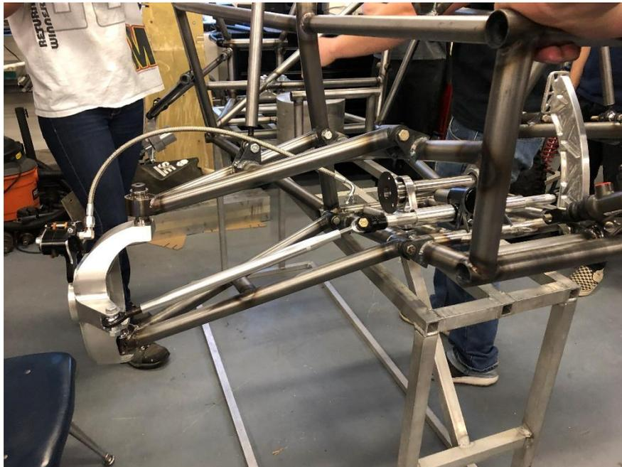
*Figure 27: Front End Assembly*
