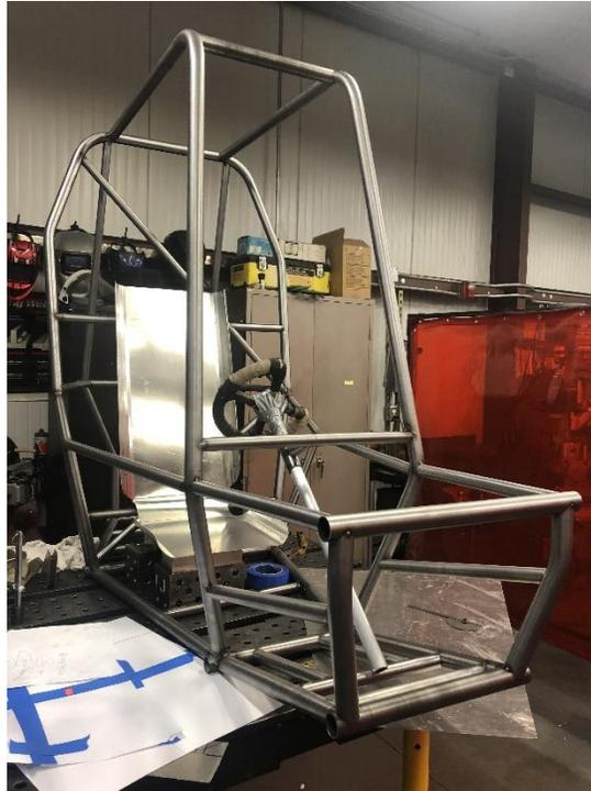
Figure 6: Front View of Frame with Complete Roll Cage and Front Members
