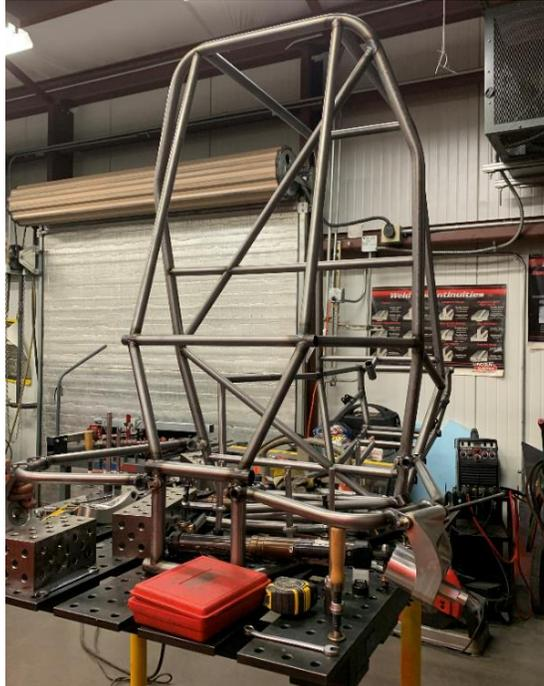
Figure 3: Rear-View of Chassis, Rear-End Shock Member
