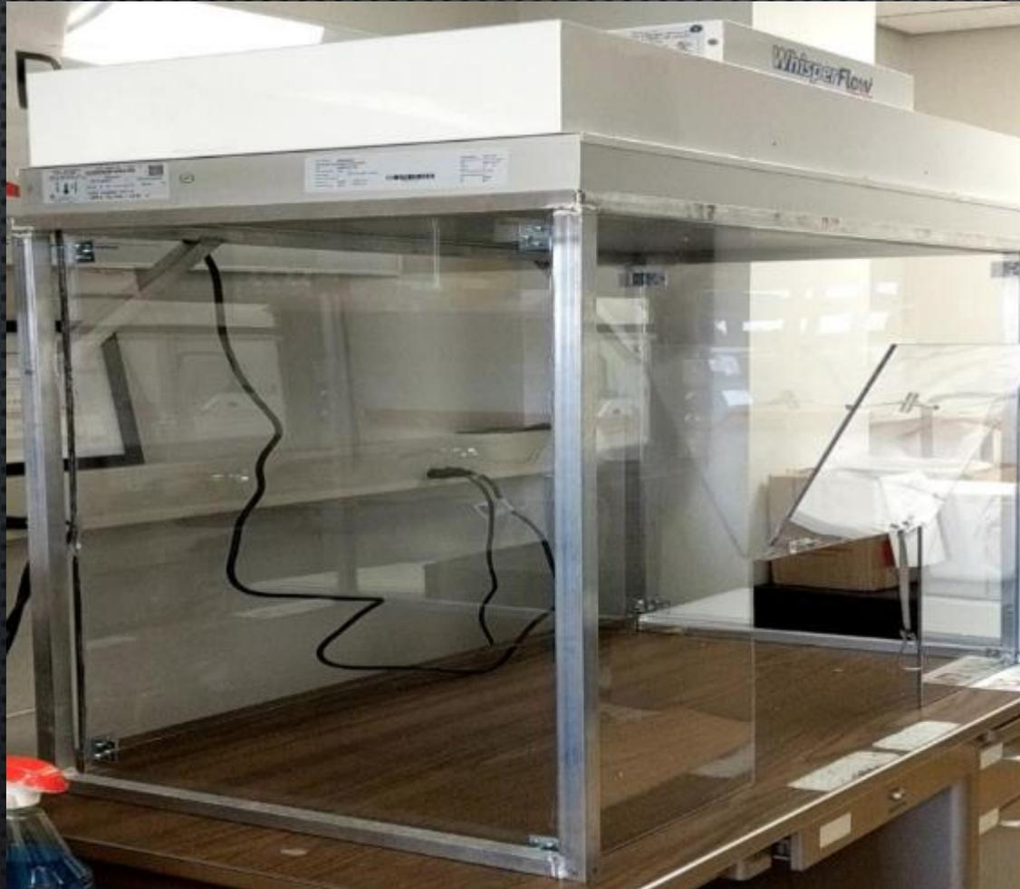
Figure 12. Finished Hood with FFU
