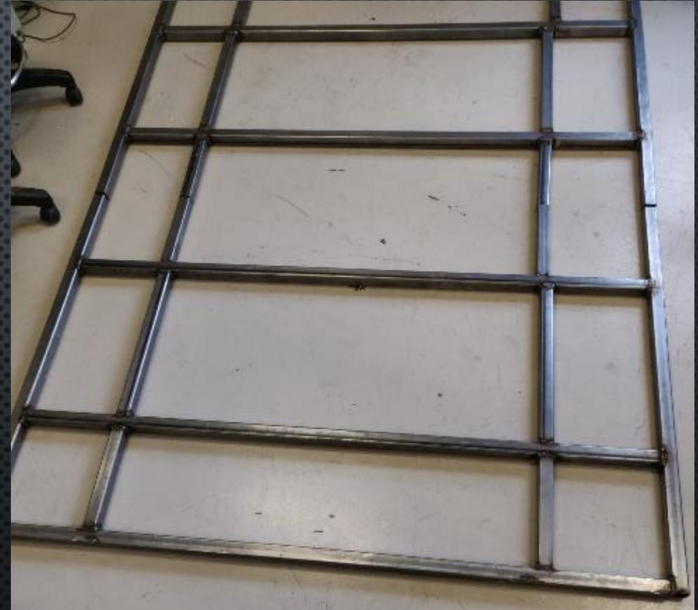
Figure 15. Welded Top of Steel Frame
