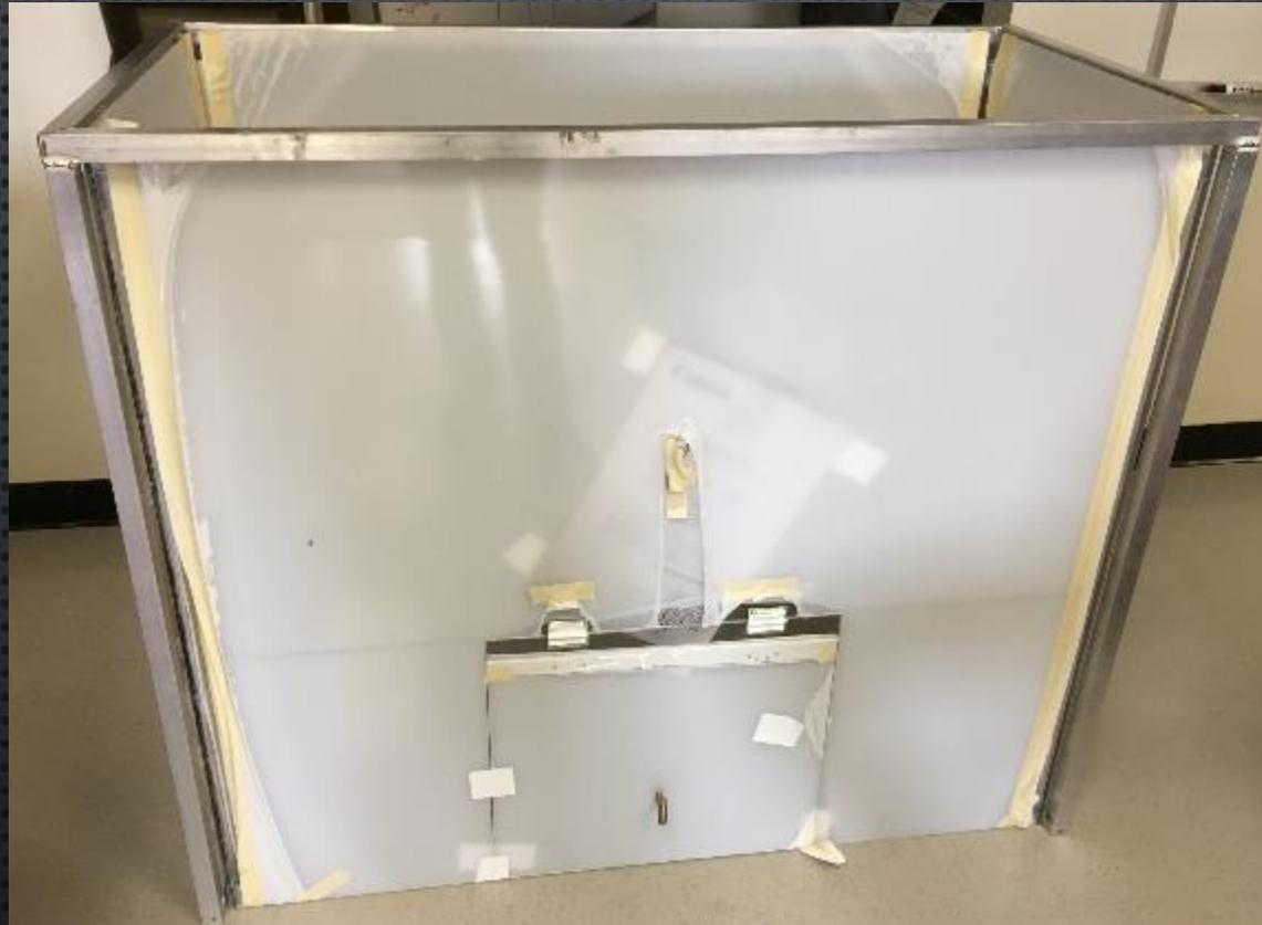
Figure 10. Finished Aluminum Frame and Polycarbonate
