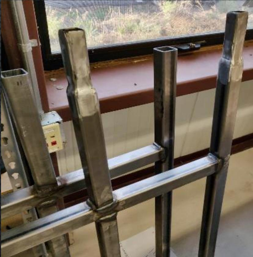
Figure 16. Telescoping Ends for Frame Top
