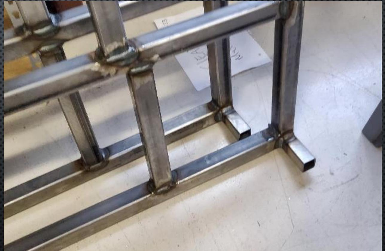
Figure 17. Telescoping Ends from Top to Support Legs
