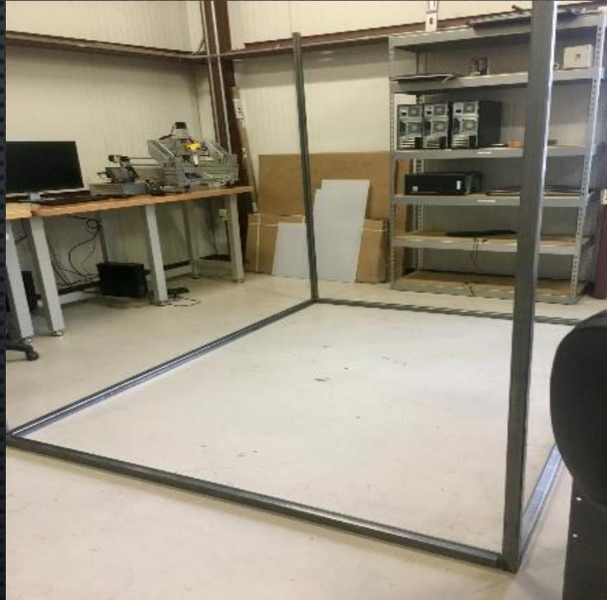
Figure 14. Legs and Supports of Steel Frame
