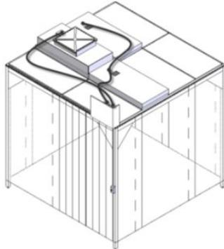
Figure 3. 8'x8'x8' Portable Clean Room [3]
