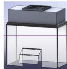
Figure 17- Portable Hood CAD Assembly
