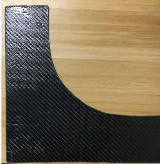
Figure 26: L-shaped carbon fiber leg support
