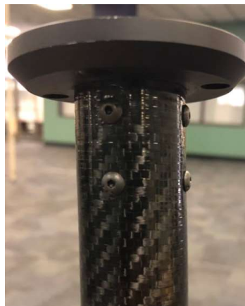
Figure 32: Carbon fiber tubing with attachment using 8 screws
