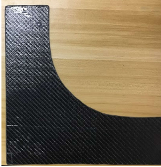
Figure 26: L-shaped carbon fiber leg support
