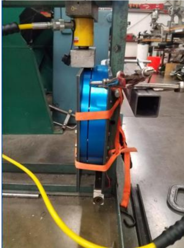
Figure 26: Shear Load Testing
