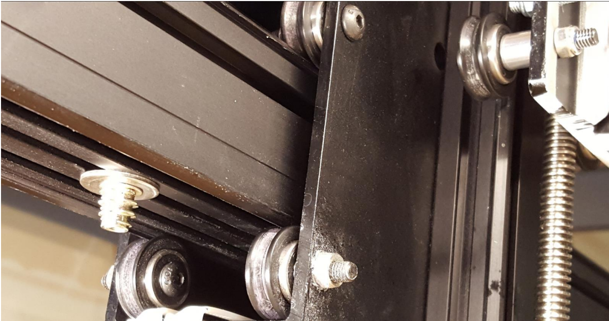
Figure 11: V track wheel system [16]
