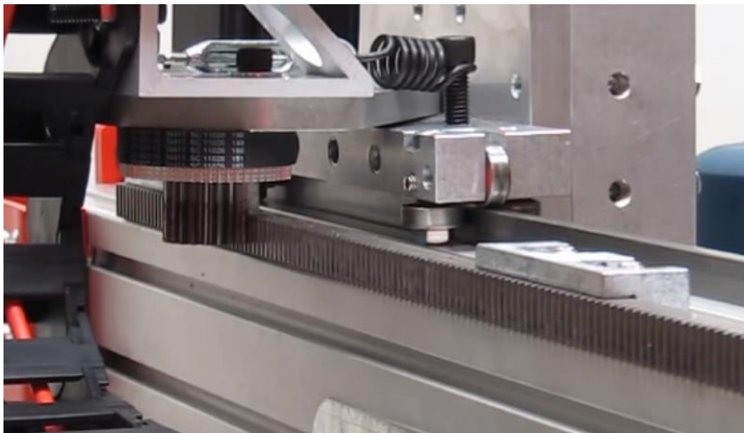
Figure 9: Stationary rack and belt driven pinion assembly [13]
