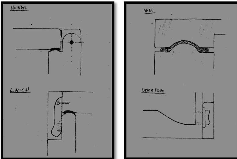
Figure 2 - Latch design (left), seal and drain plug design (right)
