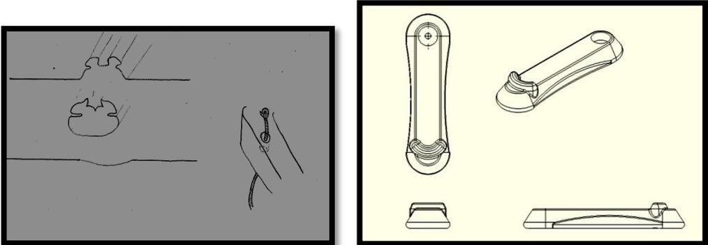
**Figure 4** - Rubber design and lock-slot and hinges (left), latch design (right)
