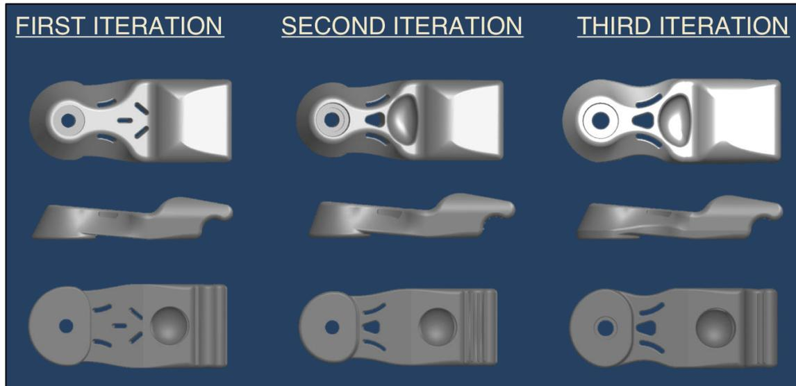
Figure 1 - Top, side, and bottom views of the three latch iterations
