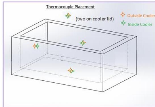
**Figure 4 - Thermocouple placements**
