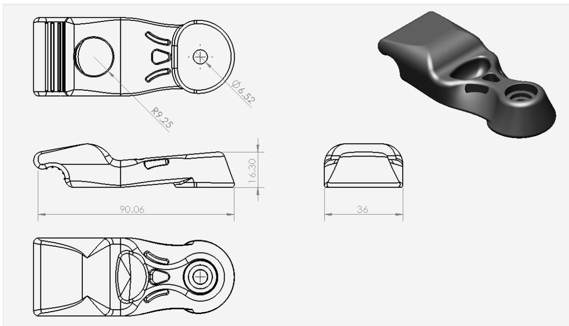
**FIGURE 18** - Design drawing for the Phantom Latch
