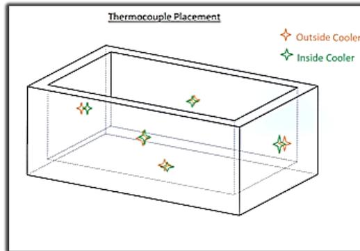
**FIGURE 16** – *Thermocouple placement for the temperature profile test*
