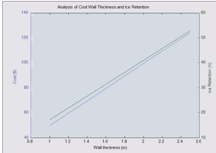
**FIGURE 11:** *Results of Wall Thickness vs. Cost and Ice Retention*
