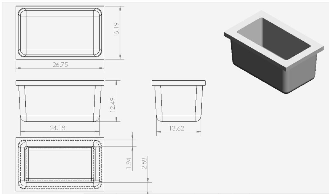
**FIGURE 17** - *Design drawing for cooler body*
