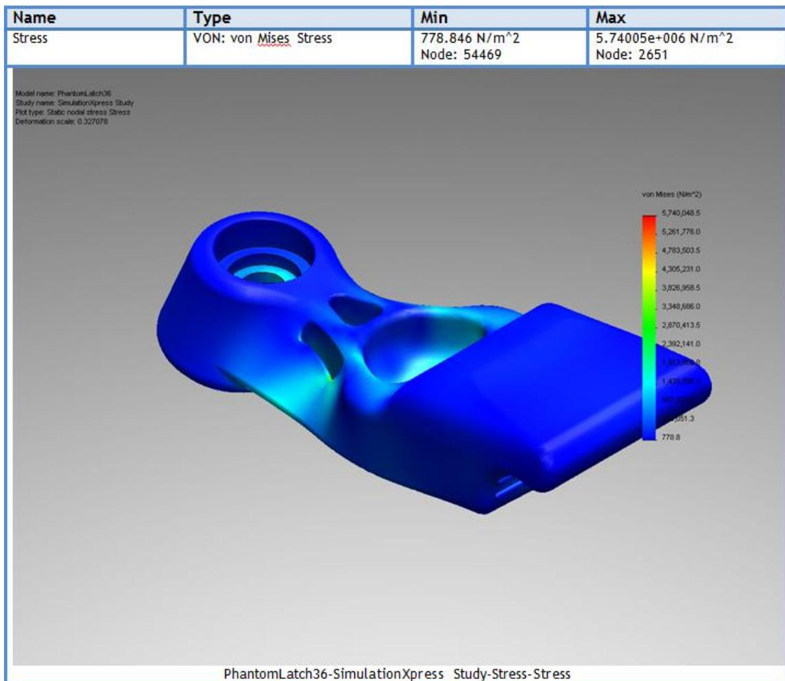
**FIGURE 19** - *Stresses observed in the Phantom Latch under a 30 lb. load.*
