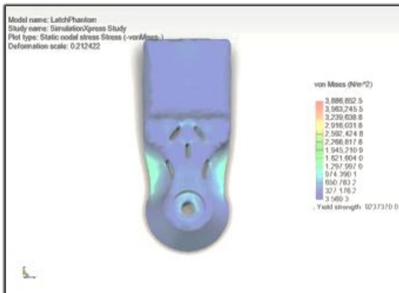
**FIGURE 12** – Top view of stress map performed on the Phantom Latch
