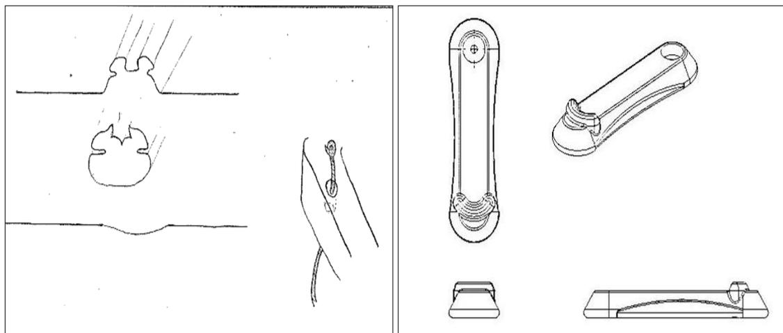
**FIGURE 7:** *Seal Design (left); Latch Design (right)*
