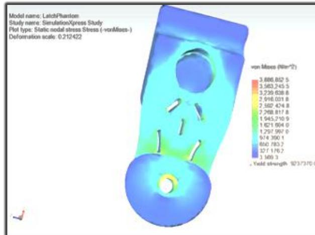
**FIGURE 13** – Bottom view of stress map performed on the Phantom Latch
