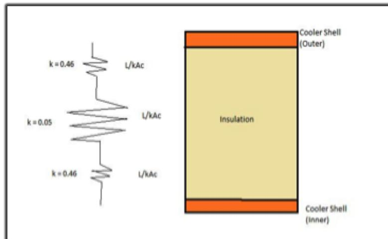
**FIGURE 10** – *Diagram and thermal circuit for cooler wall*
