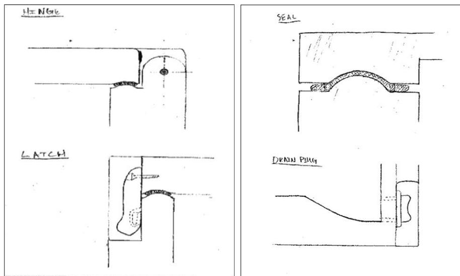
**FIGURE 5:** *Latch and hinge design (left), seal and drain plug design (right)*
