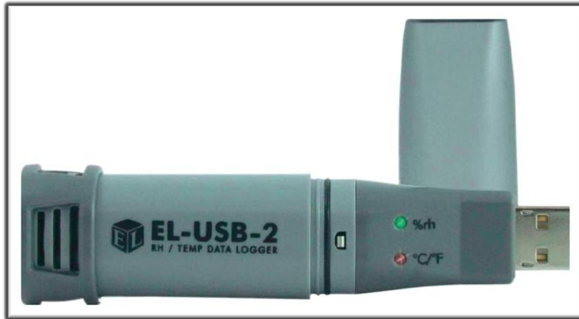
**FIGURE 14** - *Temperature data logger from Lascar Electronics [2]*
