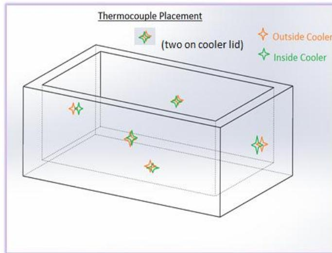
**Figure 2:** Thermocouple placement
