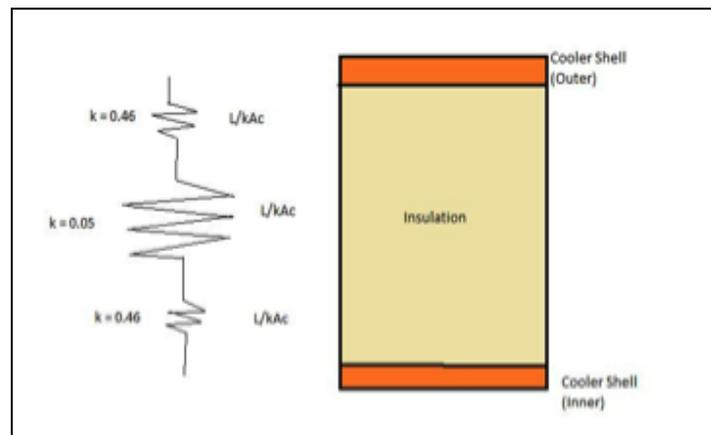
**Figure 19:** Diagram and thermal circuit for cooler wall
