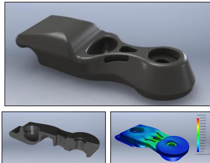
**Figure 6:** Final latch design (top), cross section of design (left), & VonMises stress map (right)
