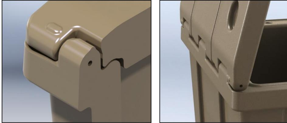
**Figure 4:** Final hinge design implementation, Cross section (left), actuation (right)
