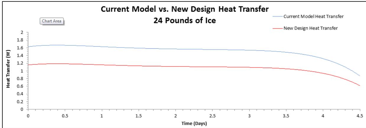
**Figure 20:** Current model heat transfer versus new design heat transfer
