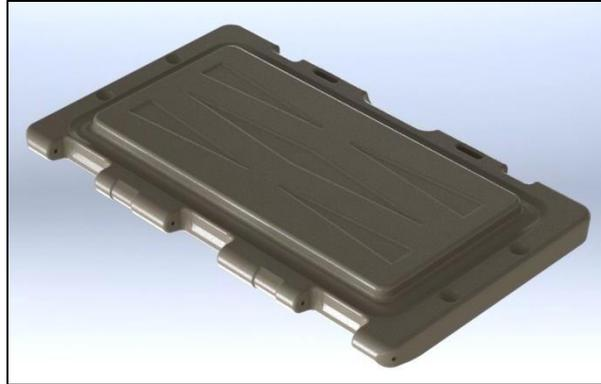
**Figure 14:** Underside of lid depicting anti-warping geometry
