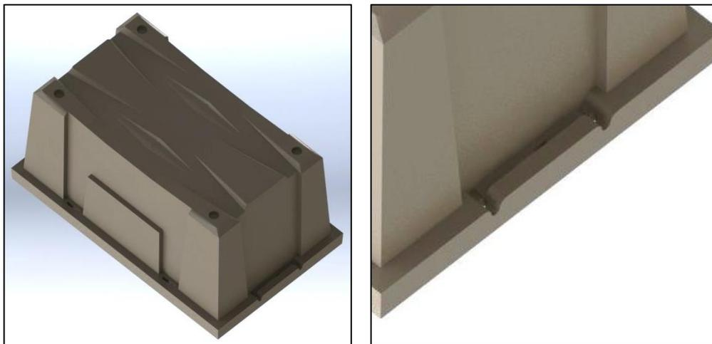
**Figure 11:** Initial Floor Design (left), Integrated Handle & Dynamic Handle Holes & Guides (right)
