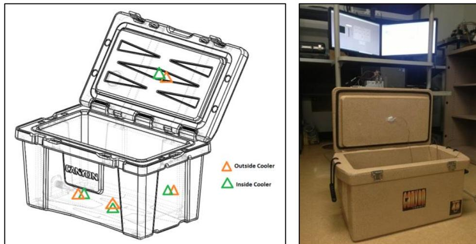
**Figure 17:** Thermocouple placement diagram (left), and experimental setup (right)
