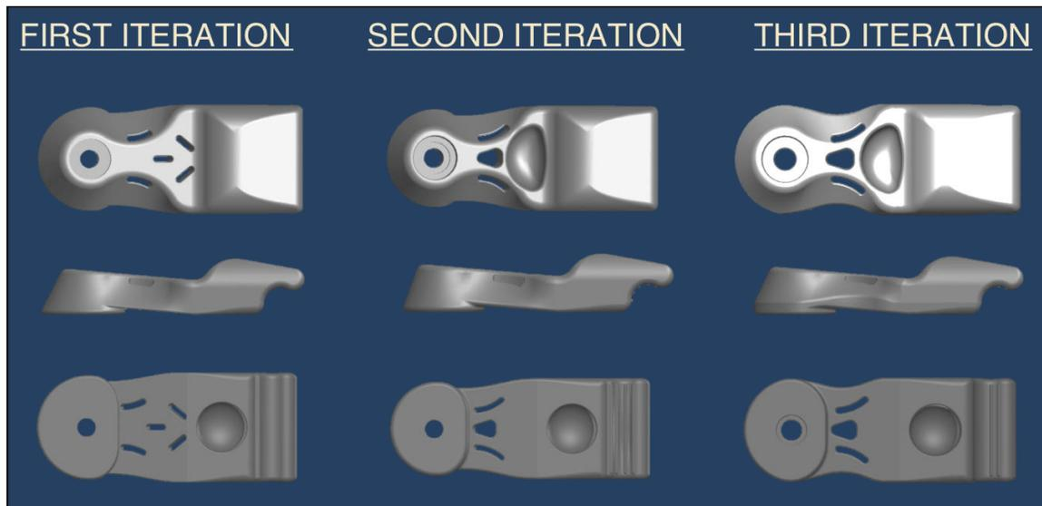
**Figure 5:** Top, side, and bottom views of the three latch iterations
