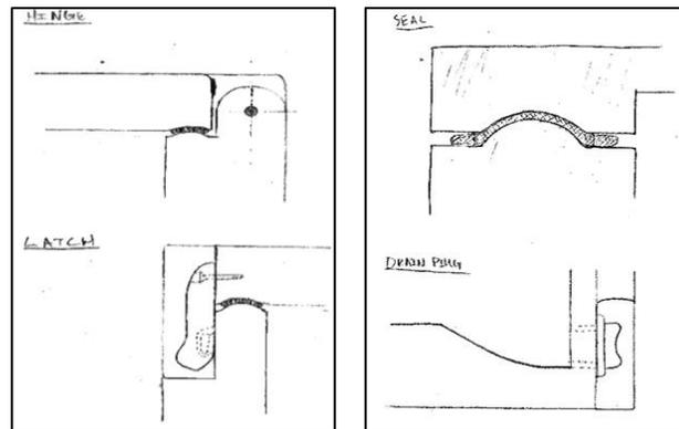
**Figure 8:** Latch & hinge design (left), seal & drain plug design (right)
