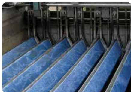
An AquaDiamond® filter with Microfiber cloth polishes phosphorus to < 0.1 mg/l.
