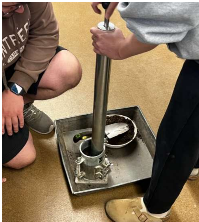
Figure 2- 8: Proctor Compaction Testing
