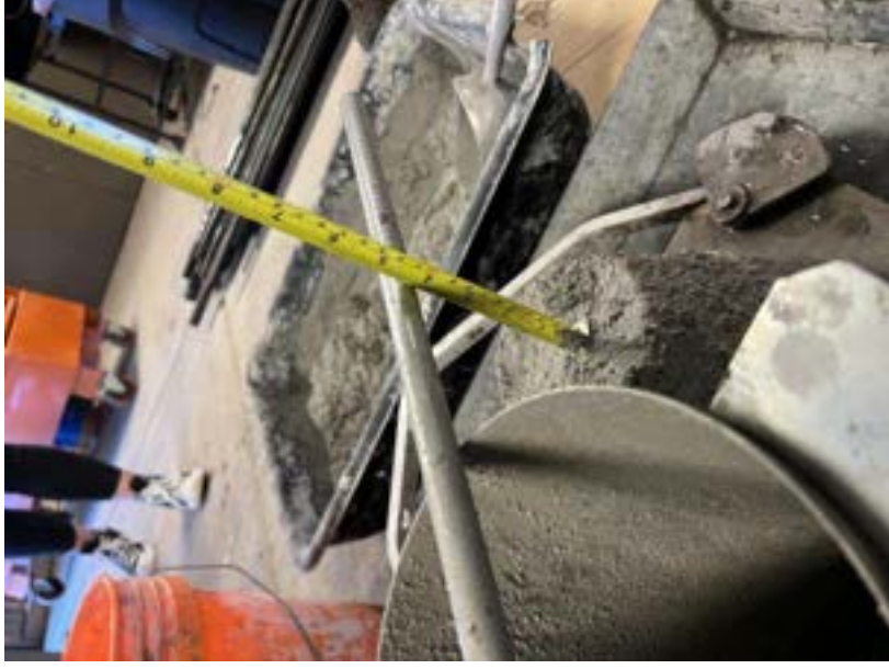
Figure 35: Slump Test (ASTM) Credit: Brendon Napier
