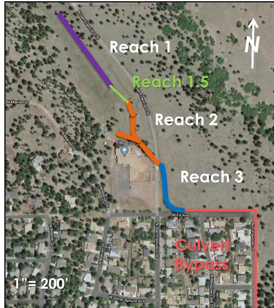
Figure 17: Switzer Wash with Natural Channel and Channel Bypass [1]
